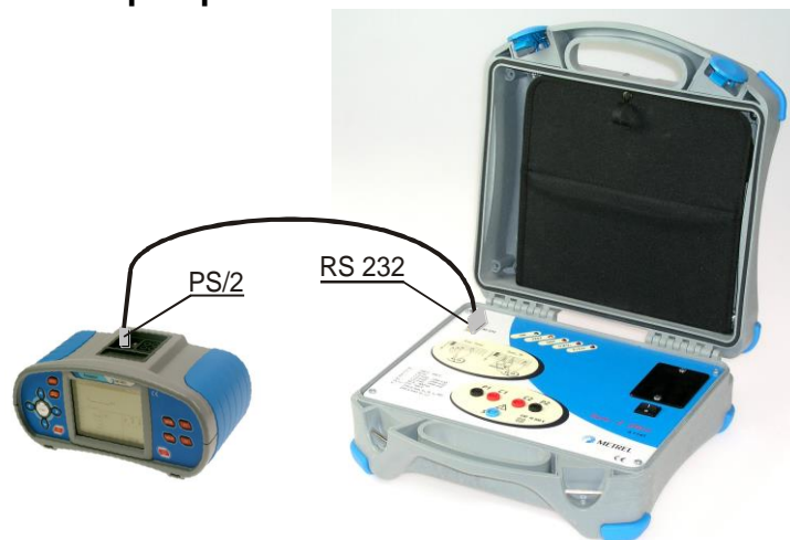
Figure 5.55: Connection of impedance adapter to the instrument
