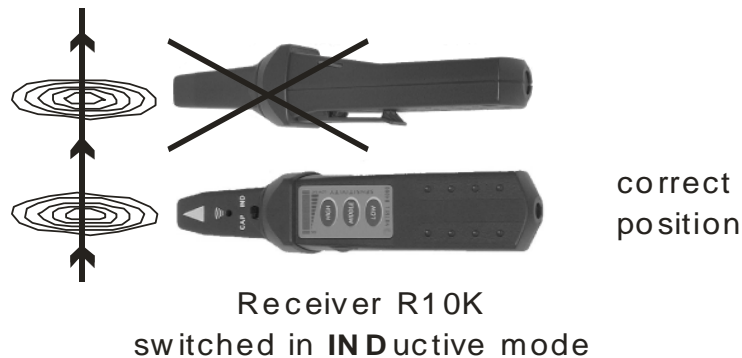
Figure C.2: Detection of electromagnetic field
